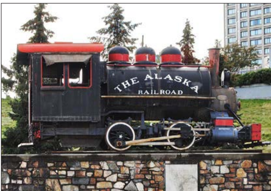
Alaska shop switcher No. 6, a Davenport 0-4-0T, was renumbered No. 1 for display in front of the depot. It once worked on the Panama Canal. photo by Bart Barton
