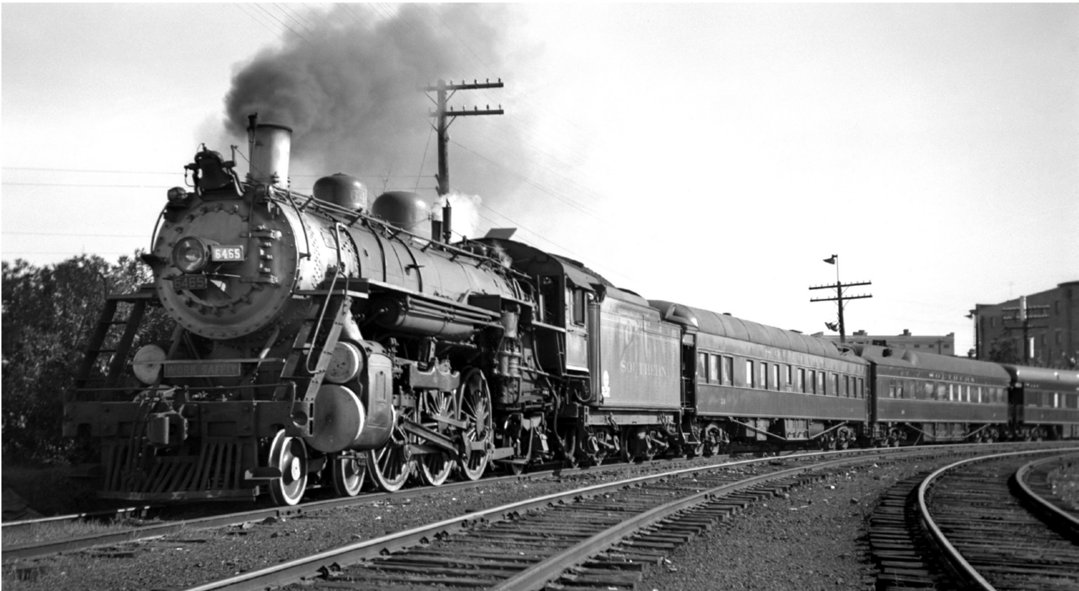
Southern (CNO&TP) 6465, a Ps-2-class Pacific, heads up a string of office cars in New Orleans, La., on Dec. 31, 1948. The panel above the pilot reads "Work Safely," and the logo at the left bottom of the tender is another safety message. (Is the purpose of this train to convey Southern officials to a meeting in New Orleans that happens to overlap New Year's Eve?) Visible are Southern wooden, steel-sheathed cars 24 and 18, and a steel AGS car. At this time, car 24 was assigned to D. W. Brosnan, General Manager-Central Lines (Knoxville); and J. S. Wearn, Chief Engineer-Western Lines (Cincinnati); car 18 was assigned to M. D Stewart, Supt. Motive Power-Western Lines (Cincinnati). Is car 16 back in the consist somewhere? ELLIOTT KAHN PHOTO, LOUIS MARRE COLLECTION
