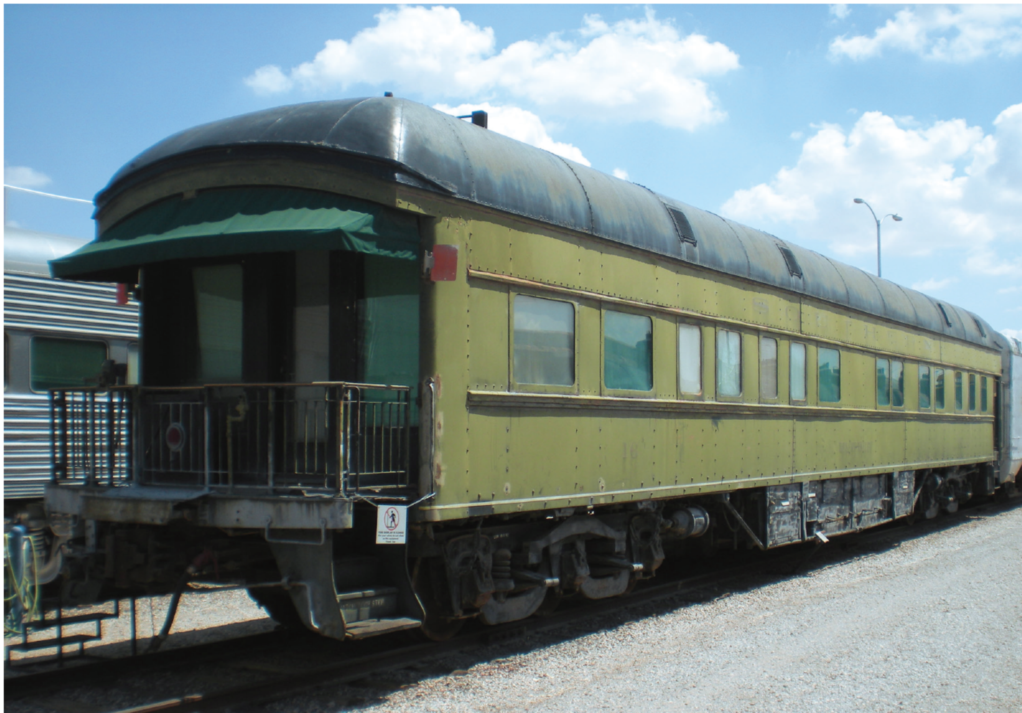
Contemporary exterior view from rear of right side of Southern 16 in Chandler, Arizona. Compare window arrangement with drawing 34-F-34: the drawing shows the seventh and eighth window from the end as being small; in actuality, the seventh window is large, and the eighth window has been removed. ARIZONA RAILWAY MUSEUM PHOTO.
