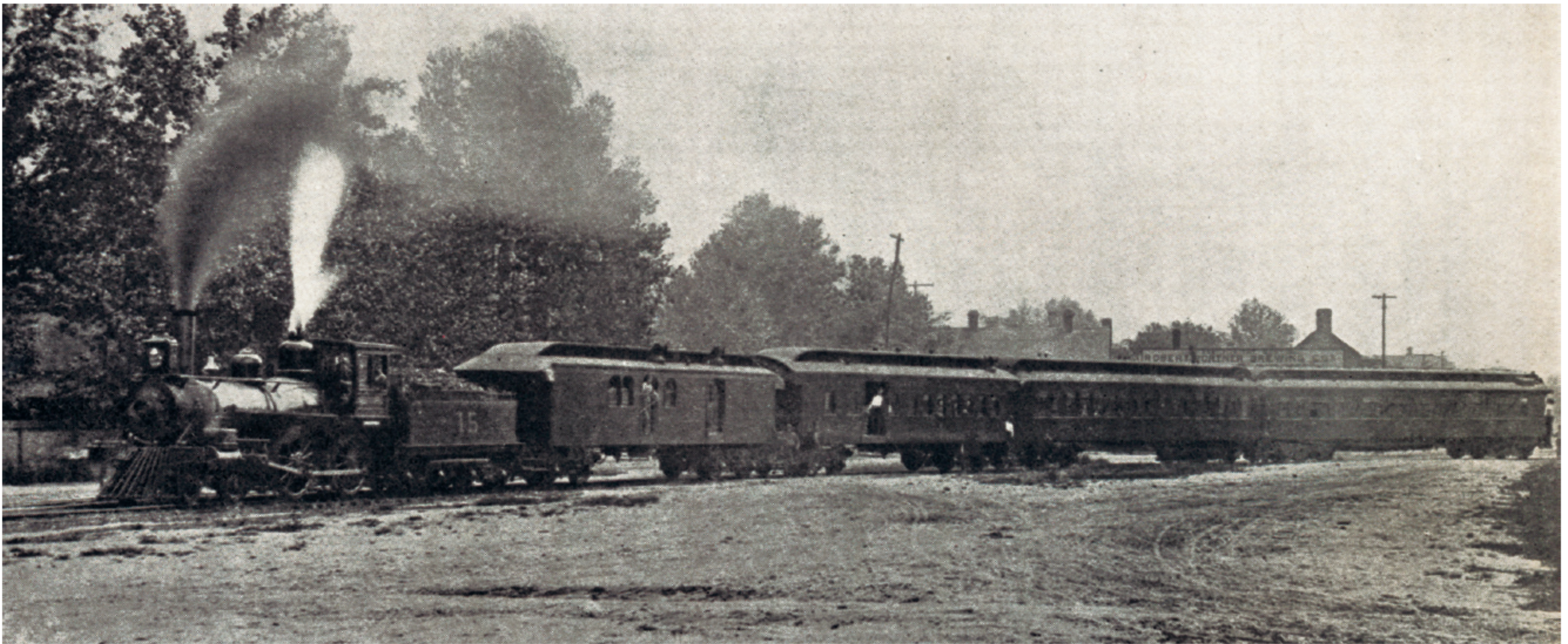
This image appeared on page 270 of Prof. Samuel Derrick's CENTENNIAL HISTORY OF SOUTH CAROLINA RAILROAD and is purported to be a South Carolina & Georgia Railway passenger train at Augusta, Ga., in 1897. The locomotive—SC&G 15, a 4-4-0—was built in May 1886 by Burnham, Parry, Williams & Co. (Baldwin Locomotive Works), originally as a wood burner. In 1890, she was converted to burn coal. The train is either No. 1 or No. 44, which were the day trains between Augusta and Charleston. The consist appears to be a full mail car, combine, and a day coach. Since the only first-class cars operated by the SC&G (and affiliates) at the time were "Palace Sleepers" running overnight between Charleston and Atlanta (and passing through Augusta either late at night or at dawn), we believe it's likely that the last car on the train pictured here is SC&G 101. Although the photo is indistinct, it appears the rear car has rectangular window frames. Assuming Interstate 101 (SC&G 100, which also exists; see sidebar) appears today as it did in 1897, it is not the car pictured here because its window frames are arched at the top. Either way, both of the office cars owned by the SC&G in 1897 survive today: car 100 in Big Stone Gap, Va.; car 101 in the Arizona desert in Chandler. SOUTHERN RAILWAY PHOTOGRAPH
