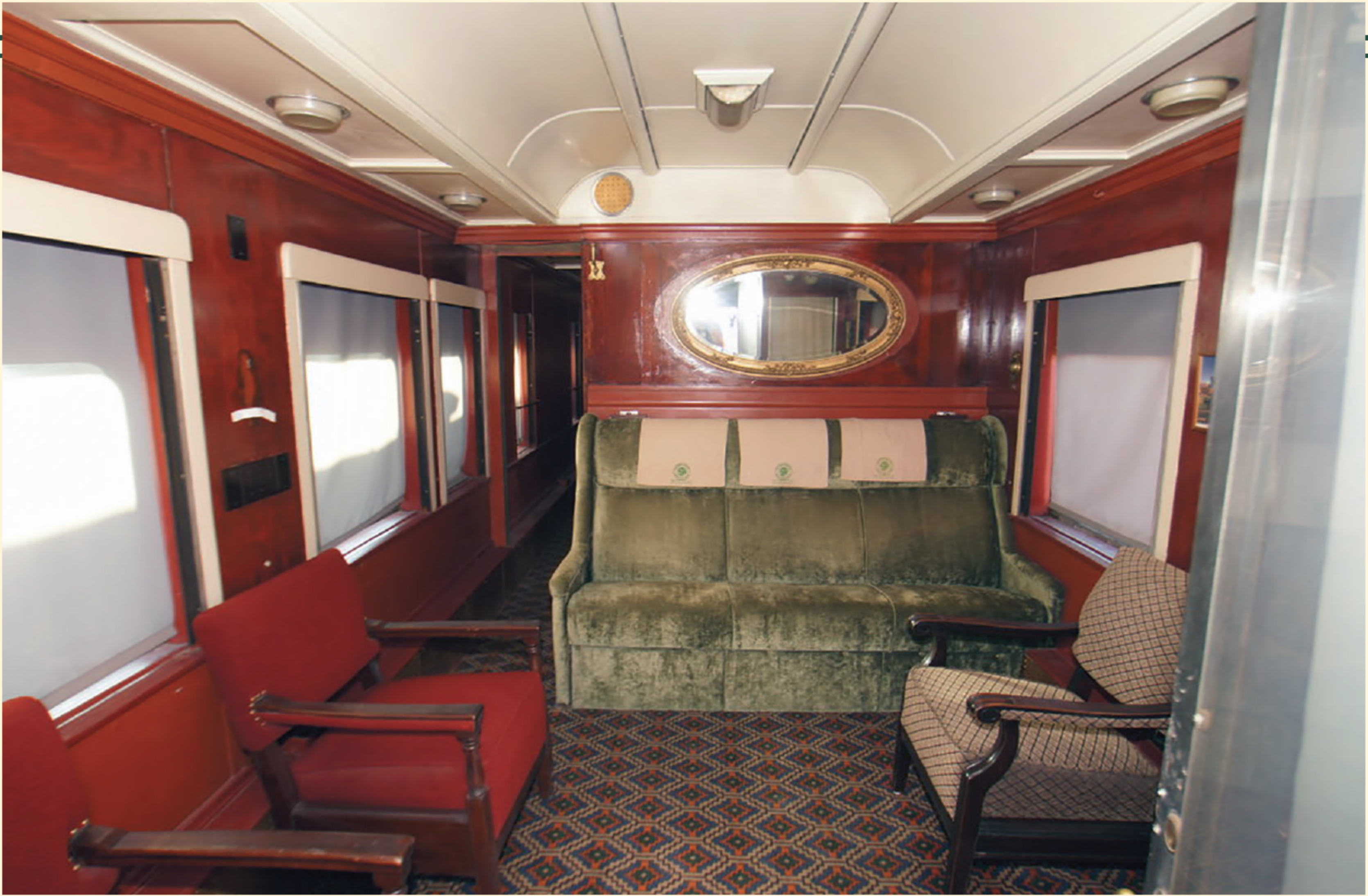
ABOVE: Contemporary view of Southern 16's lounge. The side table on the right (shown on diagram) is missing, but the sofa appears to be the kind that converts to berths.
