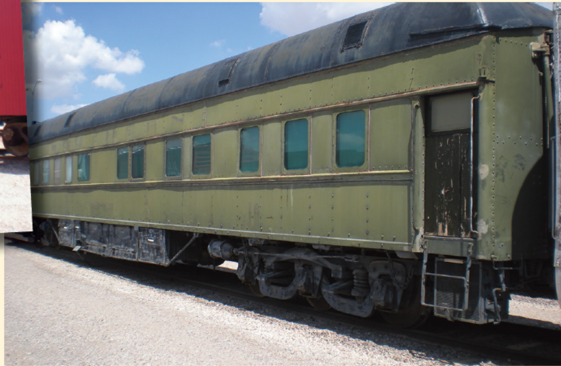
RIGHT: Contemporary view of Southern 16, right side from front. The end bulkhead window, which still appears in 1965 drawing, has been removed. Note also underbody ice boxes and monitor roof (covering clerestory), both added when air-conditioning was installed in 1939. While faded "Southern" still appears on letterboard, Desert Valley has been added on side panel in middle of car.
